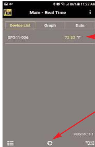
Displays the measured temperature if a probe is connected
