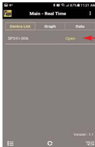
Displays Open if no probe is connected.
