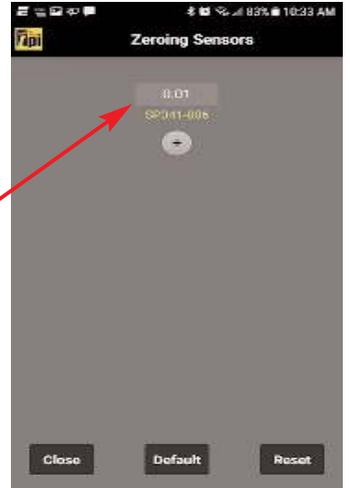
**Note:** The displayed temperature must be within  $\pm 5.4^{\circ}\text{F}$  ( $\pm 3^{\circ}\text{C}$ ) of 32°F (0°C) for field calibration to take effect.
