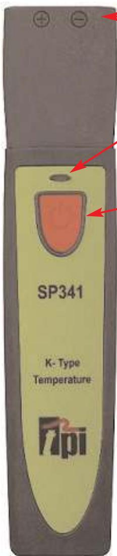
1. Input connection for K-Type probes. Connector is recessed and polarized (marked + and -). Ensure the K-Type probe is connected properly (see below).
