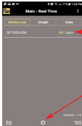
Displays the measured CO2 in ppm.
