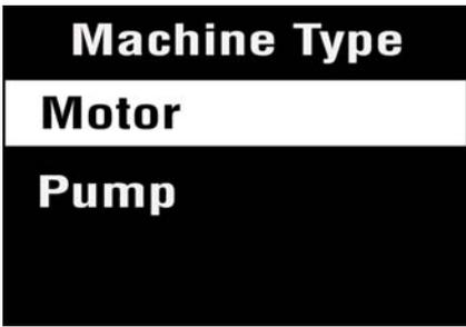
Pressing the square button again brings up the next screen which allows the machine type (motor or pump) to be selected.
