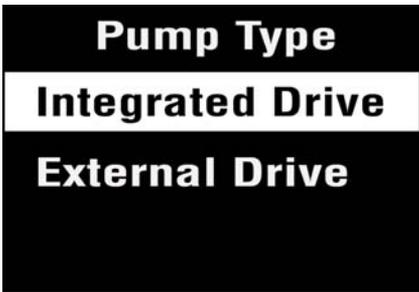
Selecting the machine type and size allows the ISO alarm levels to be set accordingly, as does specifying the type of machine mounting (rigid or flexible).
