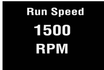
Higher run speeds may need increased BDU threshold values to identify worn or bad bearings. Lower run speeds may need decreased BDU threshold values to identify worn or bad bearings.
