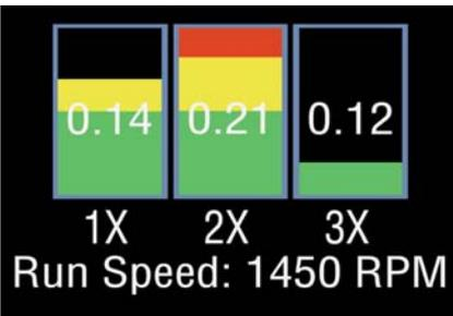
Pressing the square
